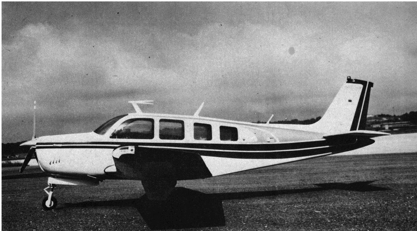
Automotive acrylic lacquer was used to give the Bonanza a prototypical high-gloss finish.
