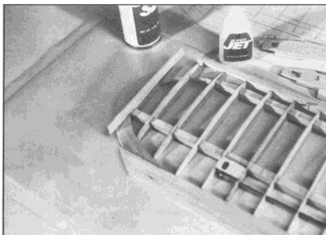
Rib R-8 added and tip ready for sanding to shape.
