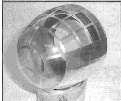
Aluminum tape intended for sealing sheet-metal ductwork was used to cover the nose and nacelles.
