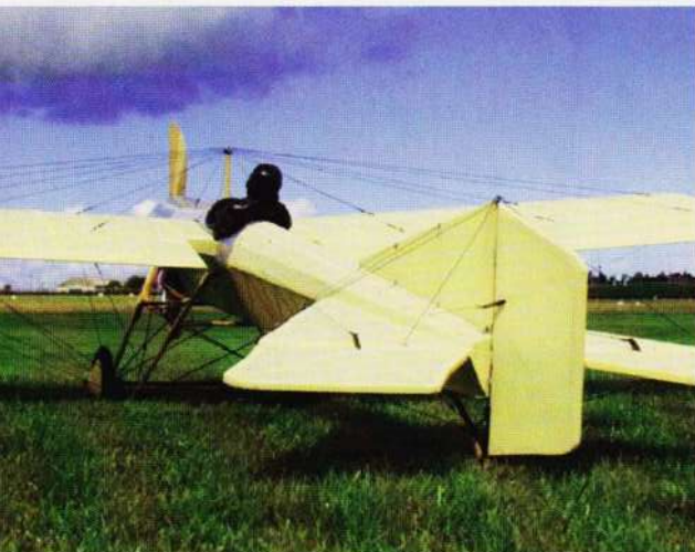
TOP LEFT: Tail feathers comprise liteply reinforcements, tinned copper wire hinges and piano wire rudder bearings.
