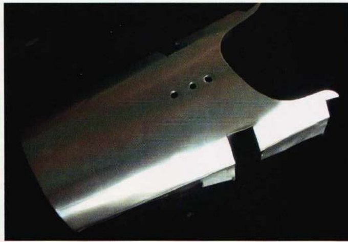
FAR LEFT: Detail of the ABS cowling and the liteply sub-cowling before the litho sheet is added.
