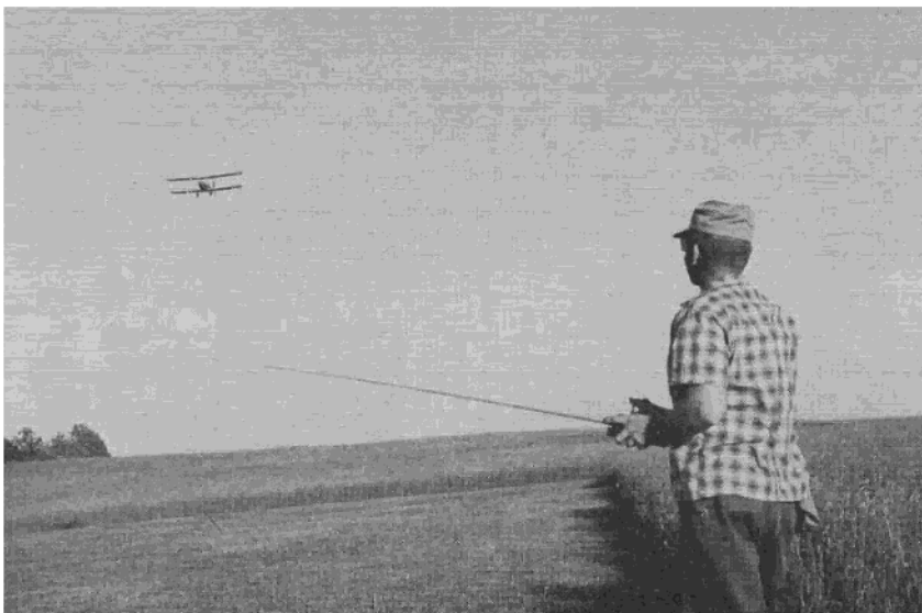
Graham Lomax and Micro-Avionics rig with Veco .61 powered Big John. With the surfaces shown, all maneuvers are very smooth, precise and unhurried. . . . The ship is extremely easy to fly, and though not a beginner's to build, is certainly an ideal ship for a beginner to fly.
