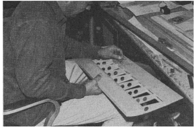
Cutting away ailerons.
