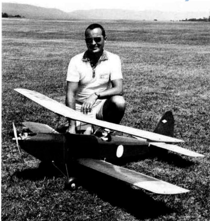
How's that for a beautiful flying field? And it's green grass, man! Note top hatch and old style cabane struts. Trexler airwheels.
