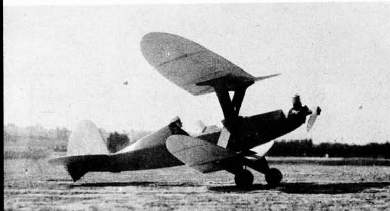
(Above) Rugged all-balsa construction does not detract from realism of Bi-Playne. (Below) "X" interplane struts support wing and fuselage. Rubber bands take shock.
