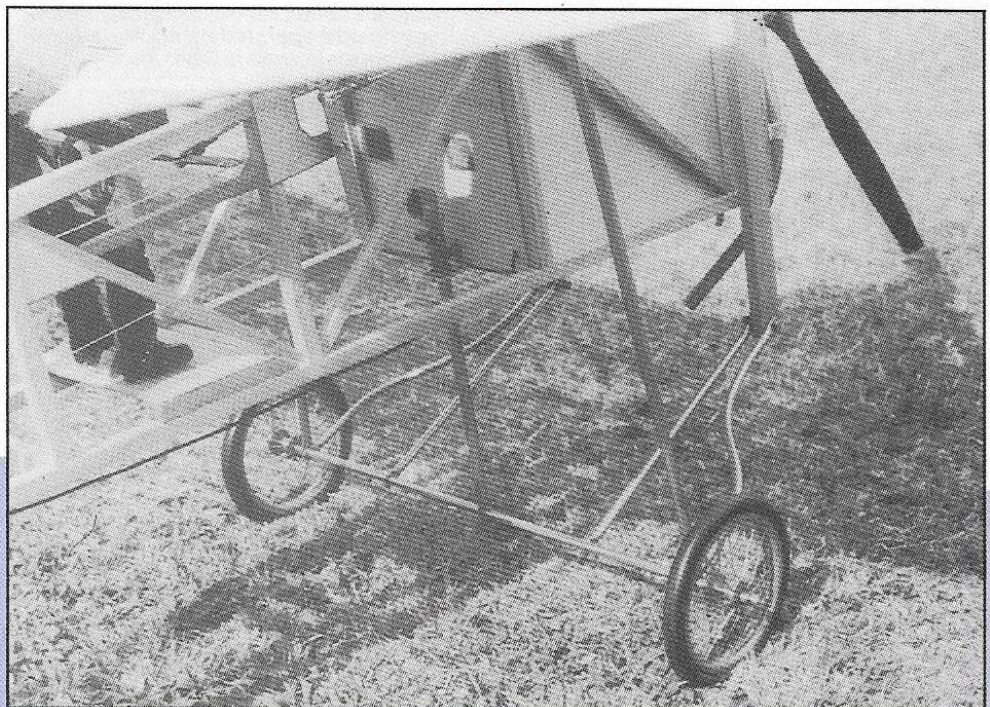
Working suspension and wire wheels give atmosphere to the Bernhardt; keen-eyed will notice a few subtle differences between pics and plan, which represents the Mk2 fuselage currently flying.
