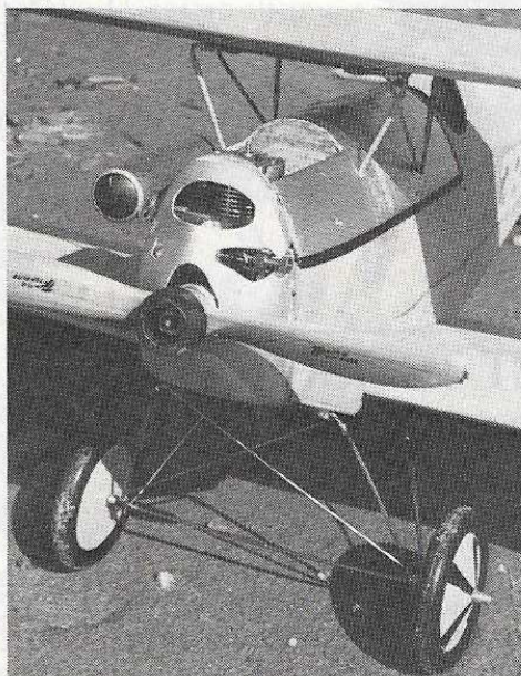
A K&B .40 cowed within, Top Flite maple prop. Landing gear is more than adequate, designed to meet the impacts. More strut work to mount the upper wing. It totals up to a rugged aircraft.
