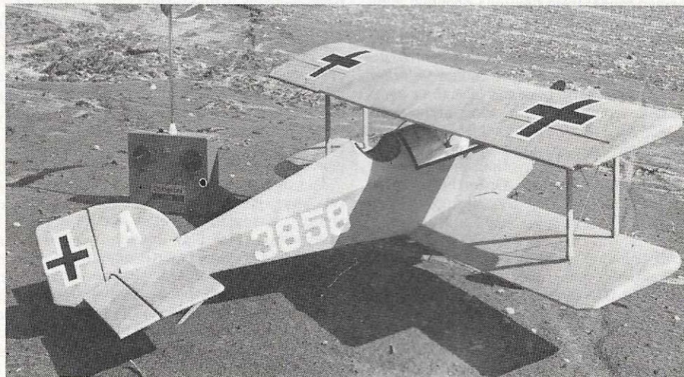
The spring-loaded tailskid. With a little luck it might drag you to a halt before the next big shell hole. Rudder horn, clevis is visible too. At top: Enough of winter, airborne at last: The ship performs nicely, fly it in for a landing. Right: Logictrol LRB-4 radio, room to spare.
