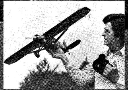
Walt Musciano proudly displays his latest control-line scale effort; note Walker U-Reely control handle.
