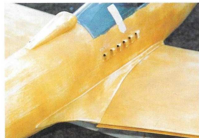
The supplied ABS wing fillets proved easy to fit and really add to the model.
