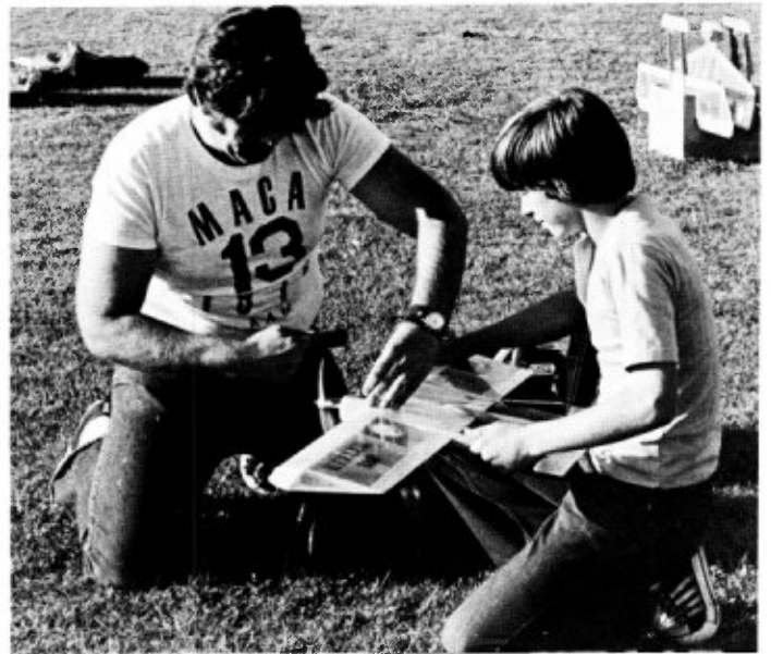
Preparing for a fast start, note size of pump used to prime the motor. Helper waits to attach battery clip and the hand flip to start.
