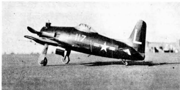
For carrier operations use a .60-size powerplant; for just scale flying without 2-speed, .35-.45 will do the job nicely.
