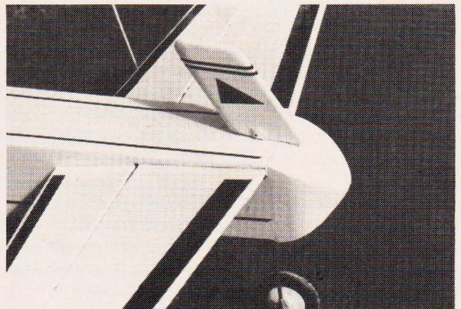
Left: Beefed bulkhead with gussets. Above: All-flying rudder seems to be in the wrong place but isn't.
