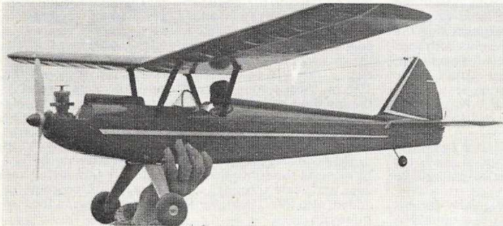
Barnstormer is an attractive single channel model which gets away from the usual boxy appearance of sports R/C model. 52 inch span machine takes a wide variety of 2.5-3.5 c.c. motors. Prototype seen here uses E.D. Racer motor, and Staveley Tone-Lock radio.
