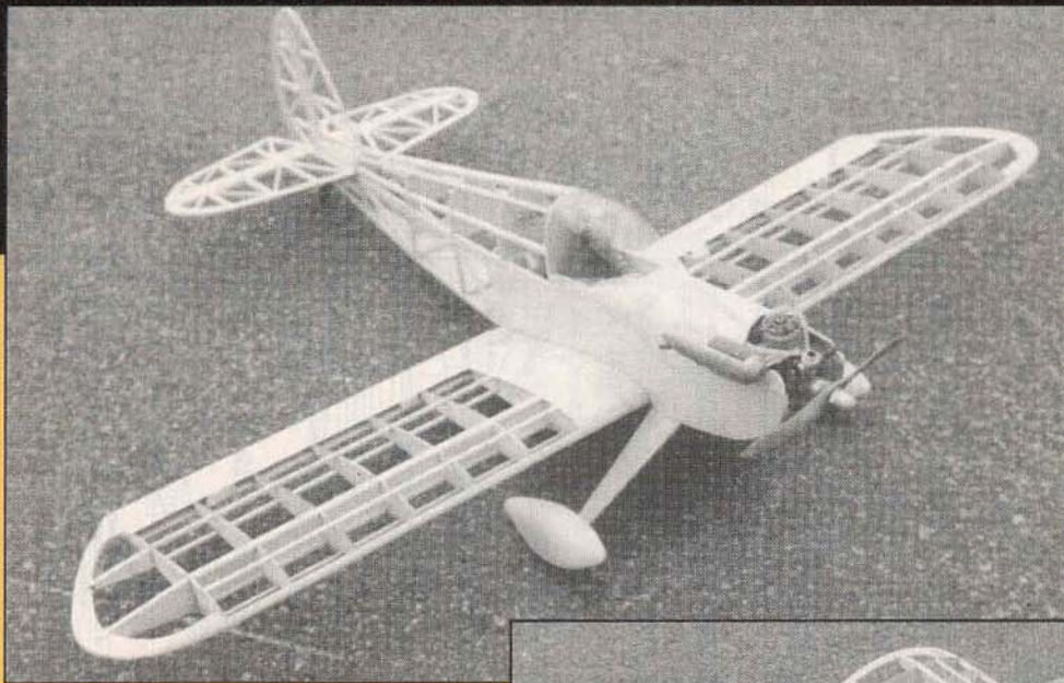
A series of framework shots illustrating light but strong construction.
