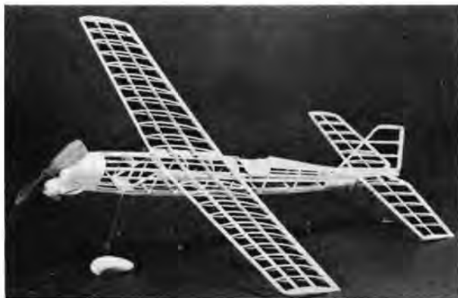
Don't let this scare you. Construction is extremely simple, with no difficult curves to contend with. Note rib construction.
