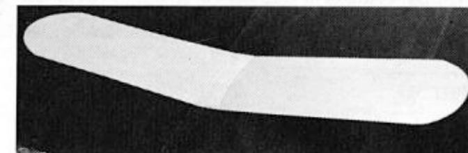
Finished wing ready for gluing to fuselage.
