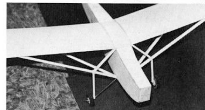
LEFT: Wing and struts glued in place. Use care when aligning all parts. RIGHT: Landing gear struts were added for looks.
