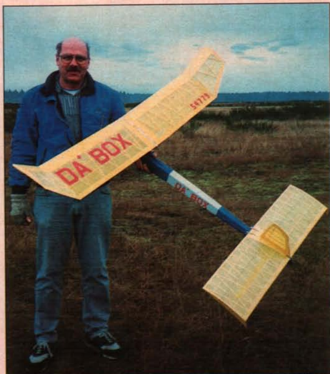
Fred Guilfoyle, who hails from the Seattle area, built two of these Nostalgia-era "Da' Box" models. This is the A/B version, powered by a K&B Greenhead. The model features a very thin undercambered airfoil wing, and climbs and glides extremely well.
