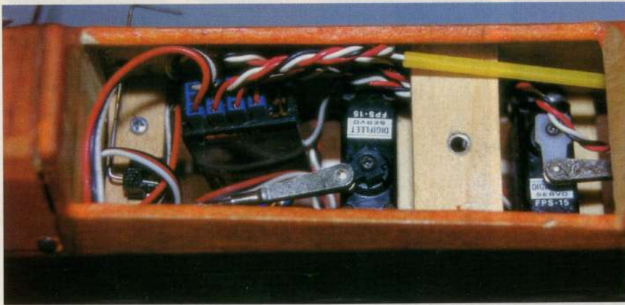
In, with room to spare! Given a bit of thought the radio installation isn't as daunting as it might at first appear.
