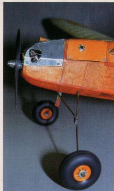
A piano wire undercarriage makes life easy during construction and has so far coped extremely well with the ruff and tumble of every day flying.
