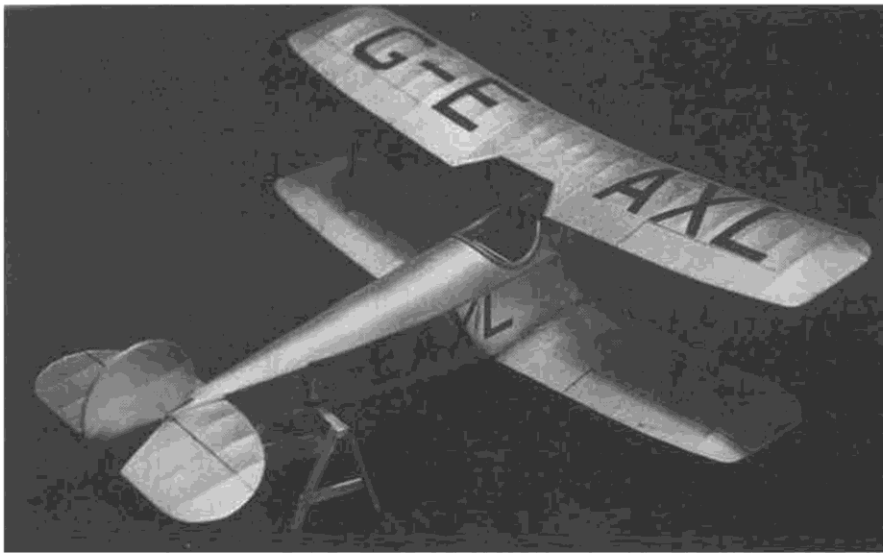
A real classy looking biplane, the AVRO is all silver with black lettering. Extremely short nose moment calls for light tail construction and a bit of ballasting.
