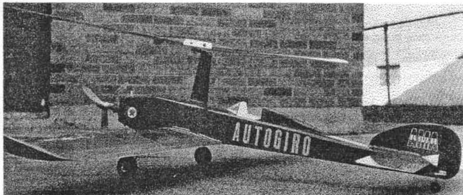
Lift created by rotor far greater than the size of rotor would indicate, very efficient.
