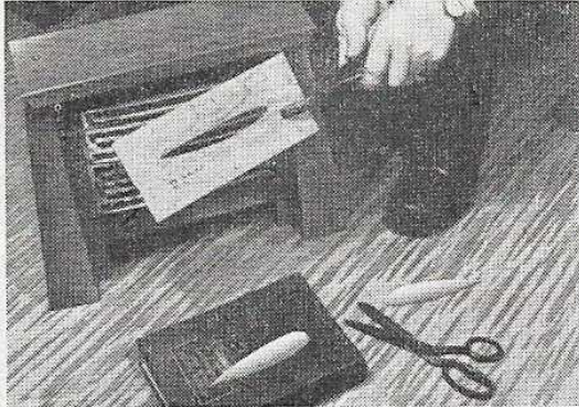
Heat acetate until floppy, with pattern ready for a quick moulding—action must be immediate to take effect
