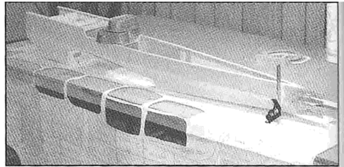
Use weights to hold fuselage in place when pulling tail together.
