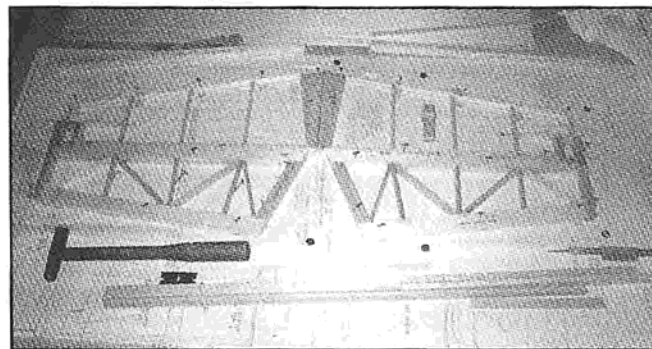
Horizontal stabilizer and elevators completed with blocks for sanding rib contour.
