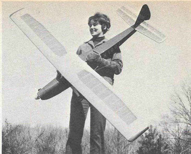
It's 25 degree weather and 25 mph winds, a typically lovely day to fly. This view shows high aspects ratio wing, long tail moment arm, both very good trainer characteristics. Wasn't easy to hold for photo in high wind.
