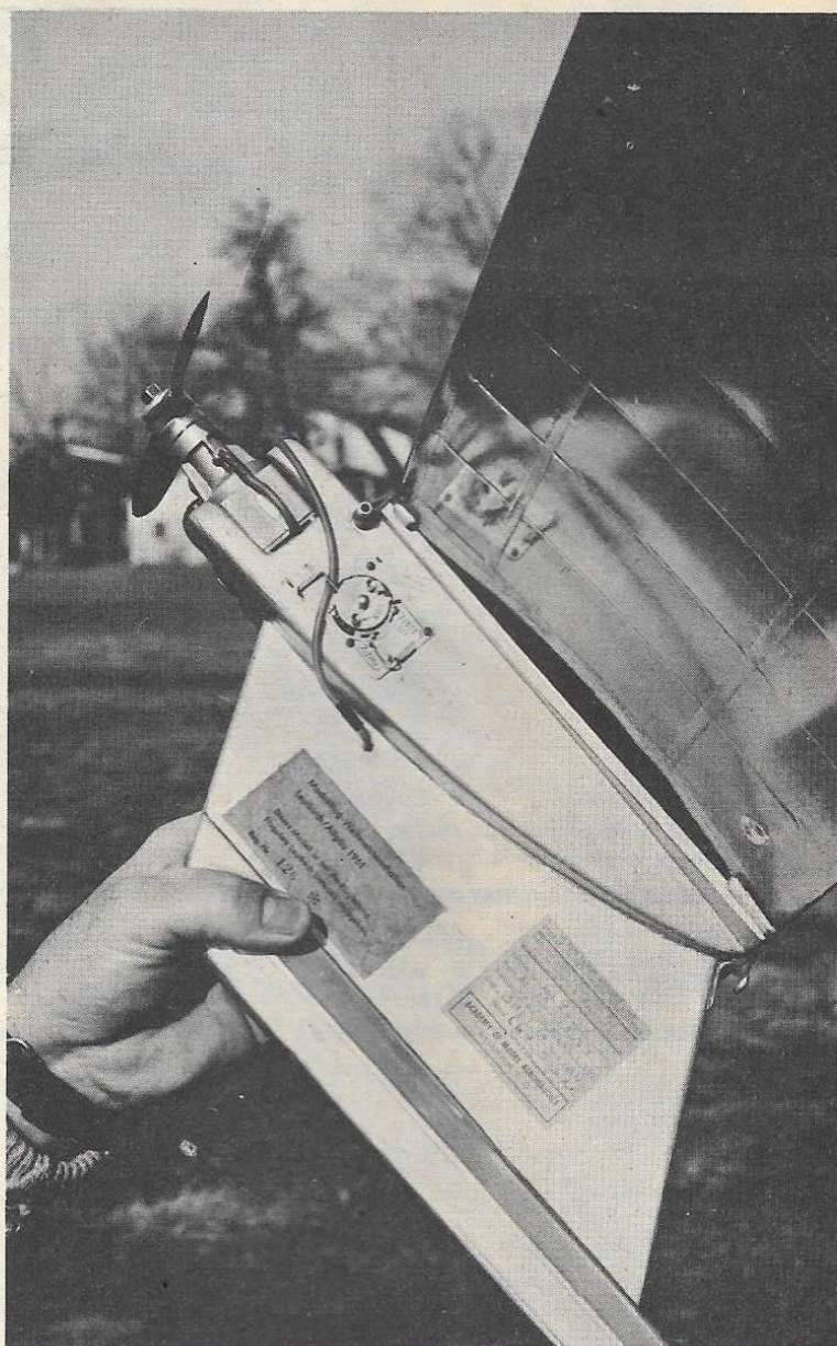
Tatone flood off timer used for motor cut-off—fuel feed lines extends through pylon from fuel tank. Note fuel pressure take-off.
