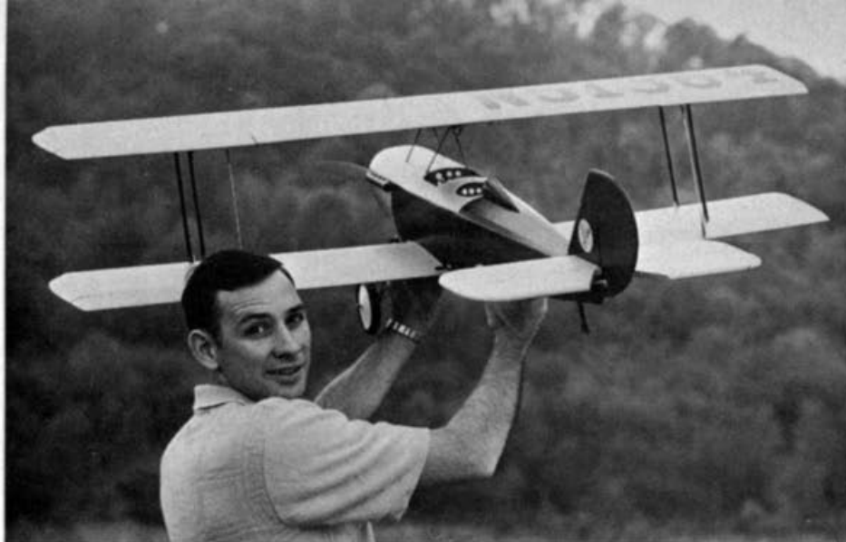
Note inter-connected ailerons, tandem cockpits. Orbit system within, flies well. Clean lines.
