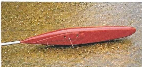
'Alto' is easily transportable and breaks down as shown at top left; designer claims he can fit three into this Metro boot! Fuselage consists of balsa pod with aluminium tube boom. Wing construction is entirely conventional and should present no difficulties. Amount of dihedral can be at your discretion; that shown on the plan makes 'Alto' a fine first aileron model capable of a wide aerobatic repertoire.
