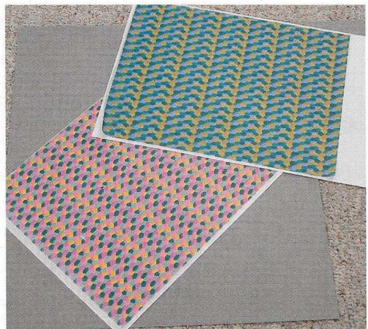
\frac{1}{16} -inch ply with balsa plug. Add a Peck thrust bearing. Printed lozenge tissue (above right). This is the way the real covering was made in 1918—pre-printed. The sheets are 11 x 17 inches. It will handle water shrinking and dopping with no problem.
