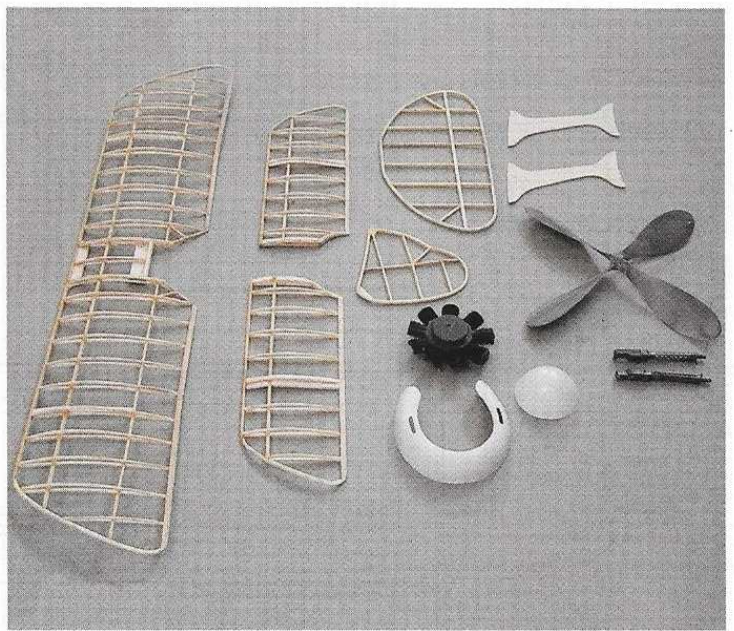
The Albatros main structure before covering. Note the sliced ribs (at left) and undercambered airfoil. The cowl and spinner (above) are vacu-formed plastic. Wing struts are light \frac{1}{32} -inch balsa. Once covered with tissue and dope, they will be much stiffer.
