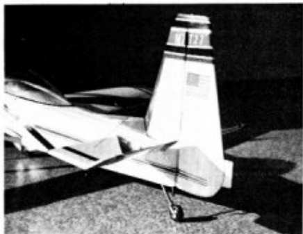
Close-up of tail section showing spring-loaded rudder, amount of elevator travel, bracing.
