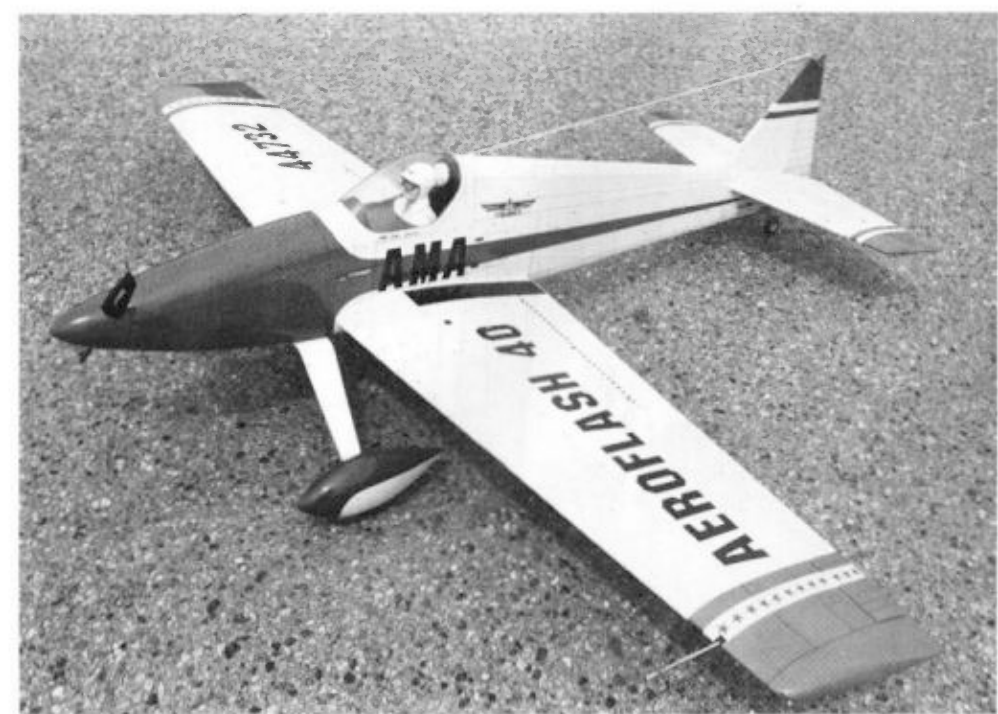
The lovely finish Ed put on the Aeroflash started with Coverite and epoxy paint. Panel lines were inked on and the Coverite lettering put on before several coats of clear were applied.
