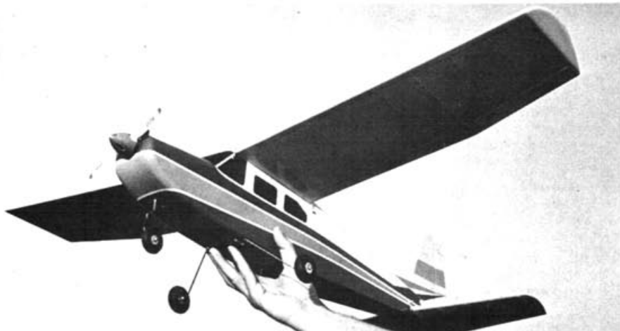
Quite a handfull Scale appearance with scale trim details, paint and striping enhance its general good looks. Nose gear has double bend knee action for absorption landing shock.
