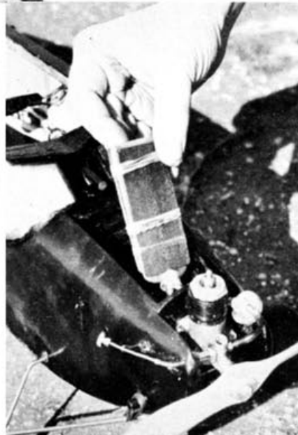
Receivers built on one side of chassis may be mounted on foam on a slip board fitting into grooves, resting against a solid bulkhead. Miller shown. Below: Left—Walker tank is folded over between ply sheets; Right—The elevator escapement and part of linkage visible at rear of the cabin.
