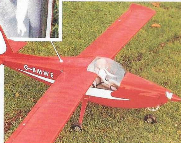
Plenty of room for cockpit detailing at 1/5 scale; span comes out at a manageable 68" or thereabouts. Easy access to radio equipment, too.
