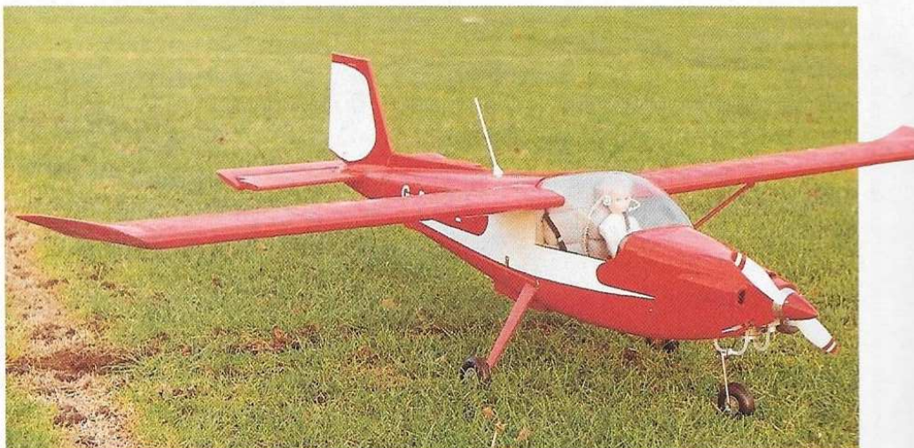
With trike u/c and simple wing, model is a perfect scale subject.
