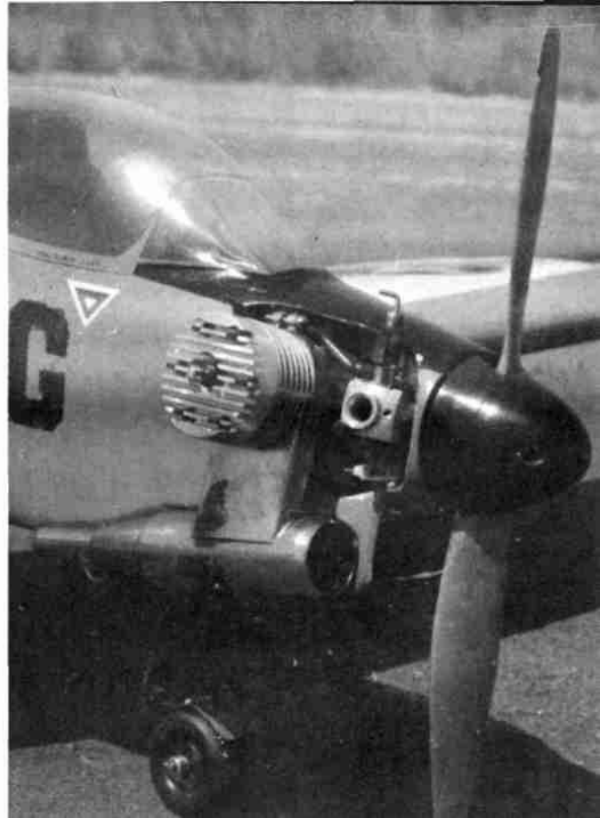
Not a tail dragger as it would seem with tail skid, this is only for those high main gear landings and touch and goes! Note rudder pushrod. Nose section showing Lee Super Custom .61 engine, slightly recessed Sil-nose encaire muffler, homemade nose wheel drag brake & Navy markings.
