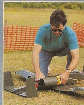
Starting the engines is easy. The leads exit the nacelle from the rear and are out of the prop's way.
