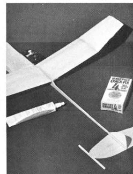
The final rigging. The stabilizer is blocked up to give it \frac{1}{8} " of tilt in relation to the wing.
